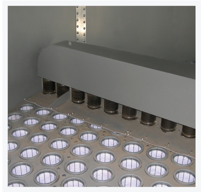
The LP cleaning arm features a flow-stop plate, which stops the airflow through recently cleaned bags to reduce dust re-entrainment
