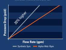
Donaldson's 10µm Alpha-Web and 5µm legacy synthetic medias are comparable in efficiency performance. The 10µm Alpha-Web allows for a 20% lower pressure drop than the legacy 5µm synthetic media. In mobile hydraulic applications where high efficiency is required but restriction is a concern, 10µm Alpha-Web provides a significant benefit to legacy 5µm media.
