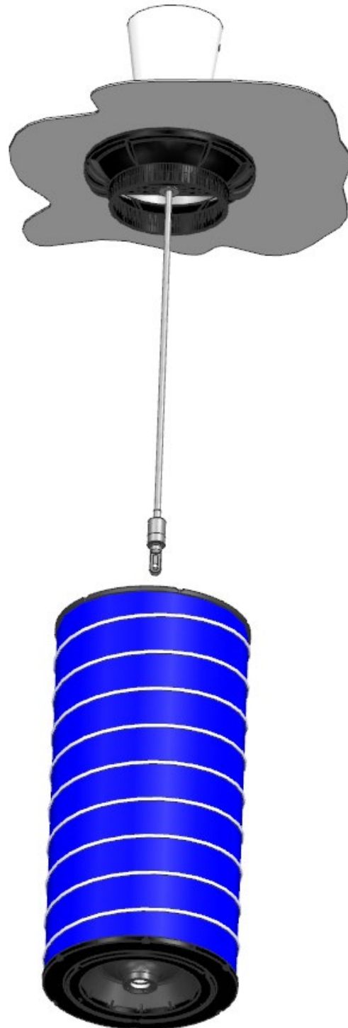
Figure 24: Installation of filter element on element support
